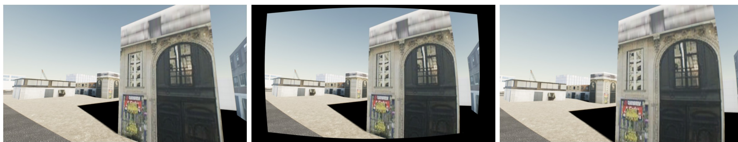
Fig. 1. (a) Undistorted 100° H-FOV image, (b) after random Brown-Conrady distortion, (c) after zoom-and-shift: invalid regions removed, geometry preserved.
